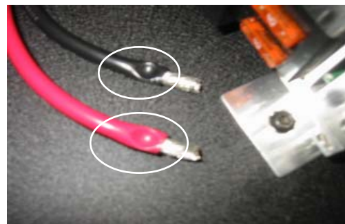
Figure 2 - Indentations on Leads
